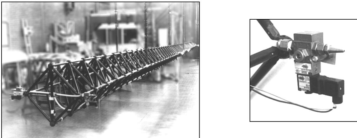
Figure 5: TESS experiment (whole view and details of one jet thruster)
