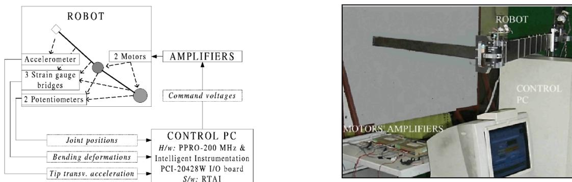
Figure 3: Block diagram and picture of the Space Robot Simulator test-bed
